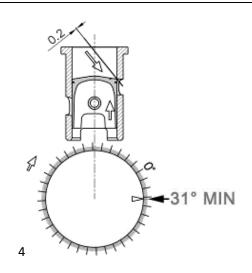
TURN CLOCKWISETO LIFT THE PISTON UNTIL IT MEETS THE FEELER GAUGE RESTING AT THE EXHAUST EDGE. AT THIS STAGE CHECK THAT THE EDGE OF DISPLACEMENTS OF THE VERNIER MATCH NOT LESS THAN **31 DEGREES.**
