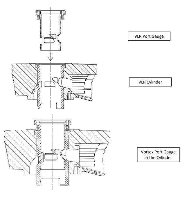
By inserting the reference port gauge in the cylinder, after having positioned it correctly, the Technical Officer will be able, at the technical scrutineering, to detect any irregularities.
