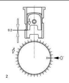
TURN COUNTERCLOCKWISE AND LOWER THE PISTON UNTIL IT MEETS THE GAUGE RESTING AT THE EXHAUST EDGE, AT THIS STAGE SET THE SCALE ON THE POSITION OF O DEGREES.
